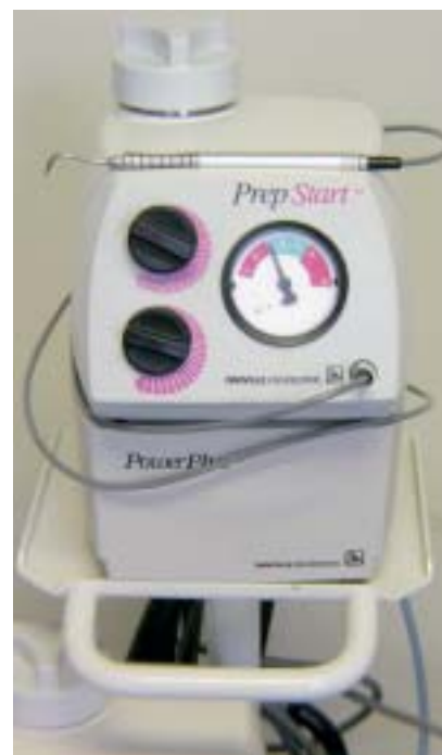
Fig 3 The preparation unit including the booster, which raises the air pressure up to 9 bar.
